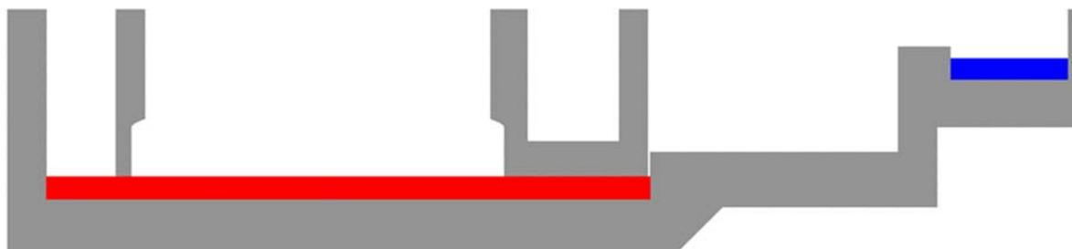
Figure 10: Final state of the wet storage building for the 1.5 MW case after 300 days of accident progression (red: corium, blue: water)
