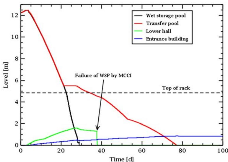
Figure 7: Water levels in wet storage building for the 1.5 MW
