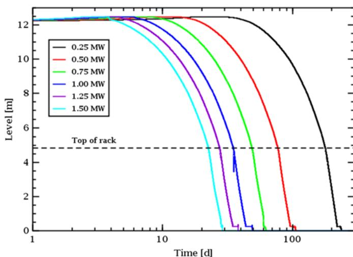
Figure 4: Water level in wet storage pool for base cases with different heat load
