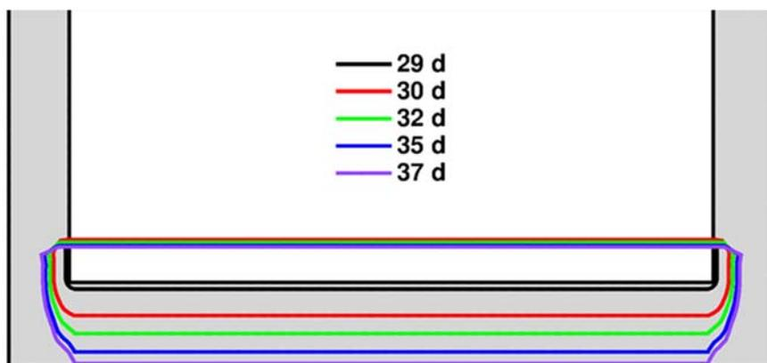
Figure 8: Core-Concrete-interaction in wet storage pool for the 1.5 MW case after melting of the steel liner
