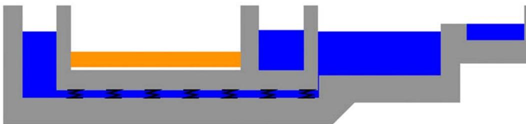
Figure 6: Final state of the wet storage building for the 0.25 MW case after 300 days of accident progression (orange: debris, blue: water)
