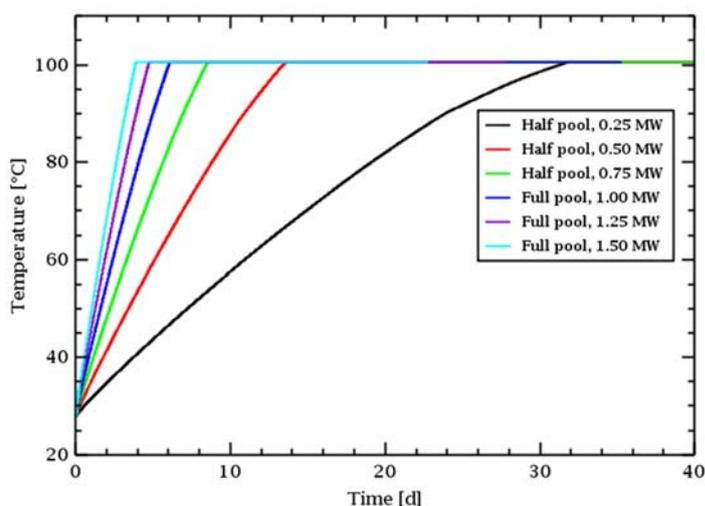
Figure 3: Temperature history of pool water for different heat load of the spent fuel
