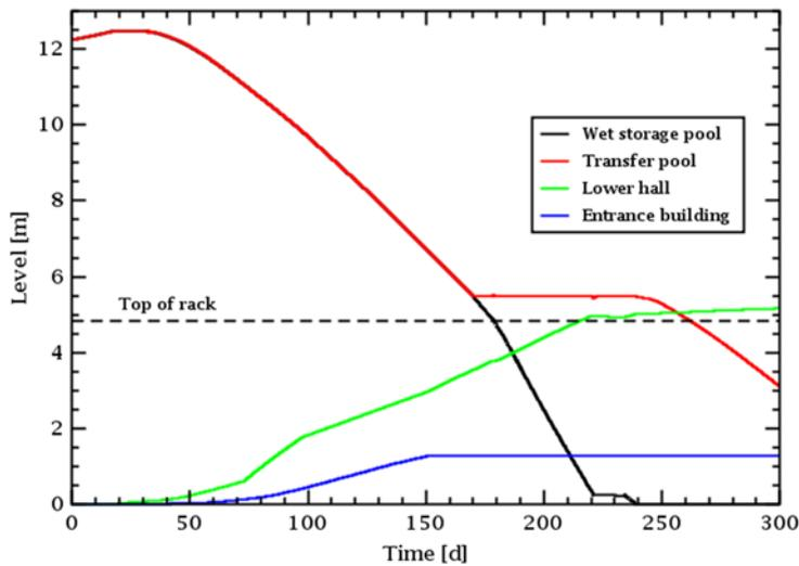
Figure 5: Water levels at different locations in the wet storage building for 0.25 MW case
